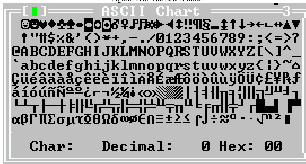
Figure 6.18: The ASCII table
