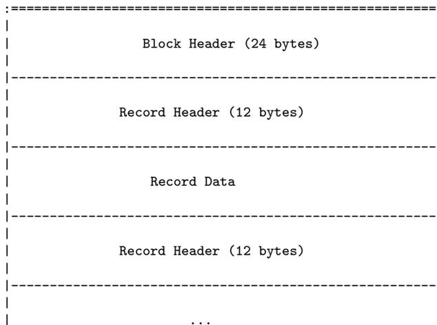
Block Header: the first item in each block. The format is shown below.
