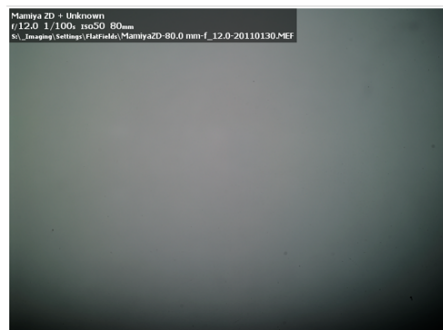
The same flat field image shown with exaggerated contrast and saturation to visibly demonstrate color and luminance non-uniformity due to the lens cast effect
