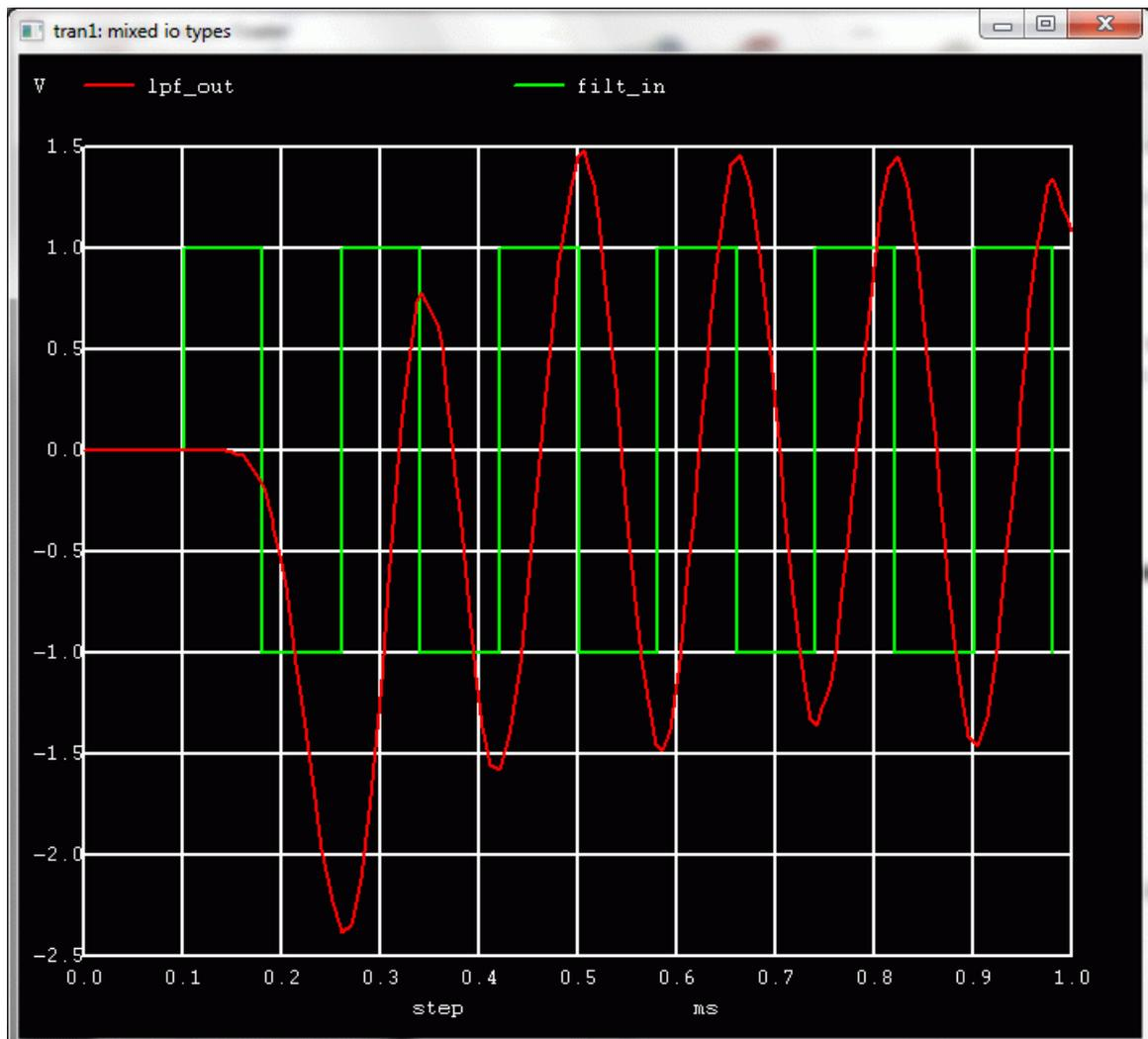
Figure 25.3: Nutmeg Plot of Subcircuit Internal Node
