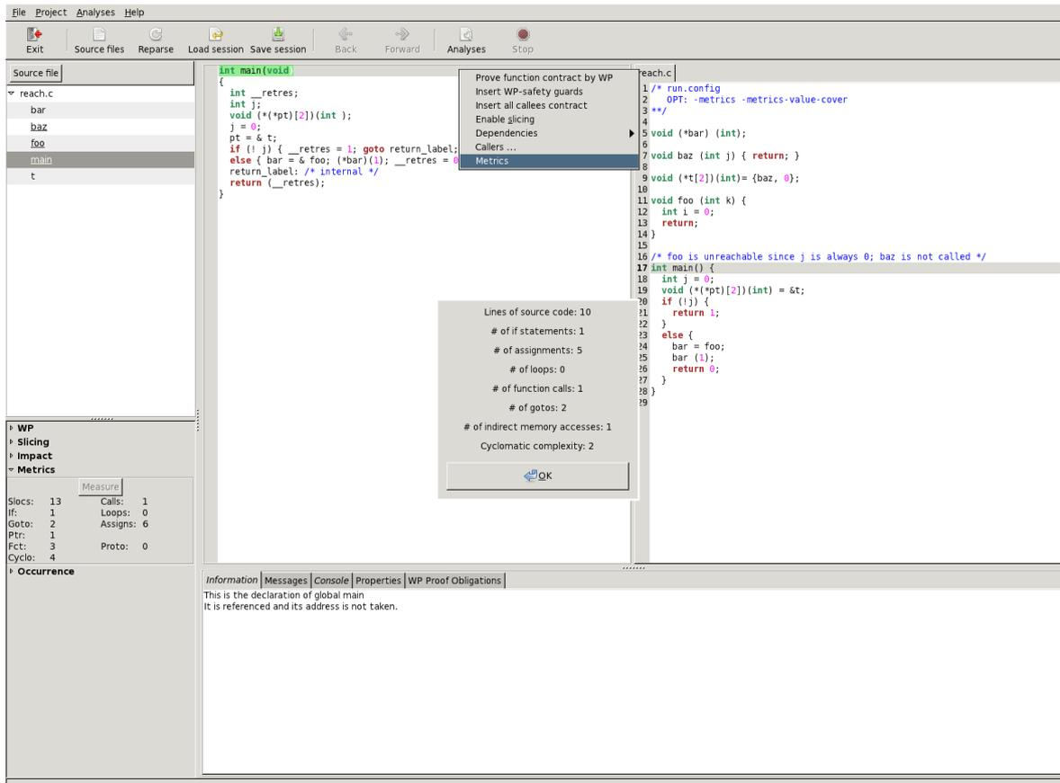
Figure 1.5: Metrics GUI: calculate metrics for a function
