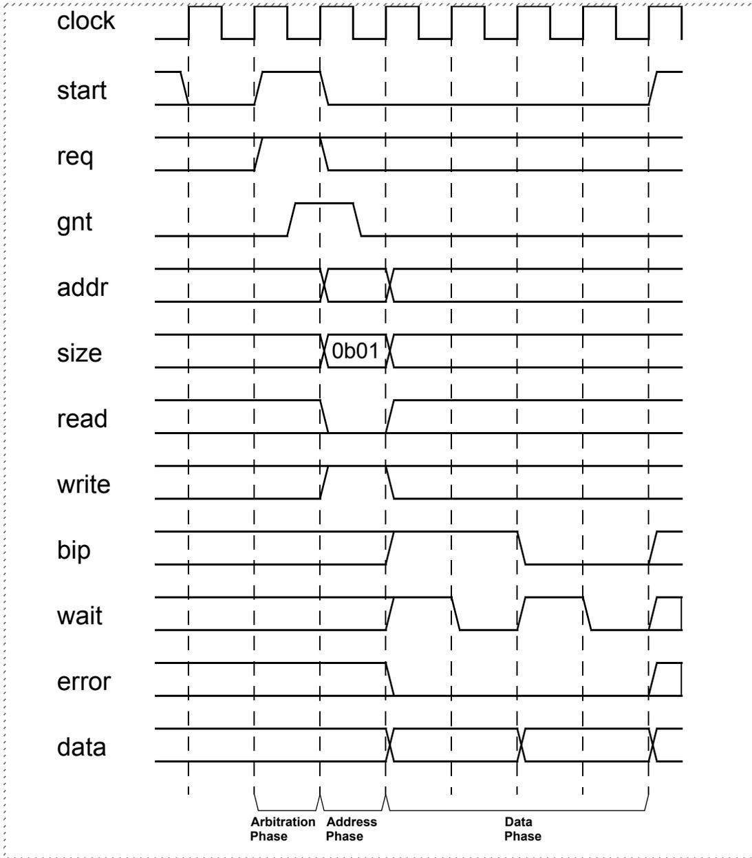
Figure 7-2 Example Read Waveform
