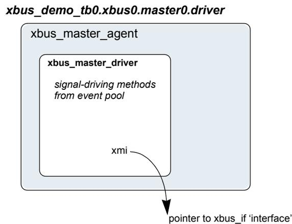
The primary role of the driver is to drive (in a master) or respond (in a slave) on the XBus bus according to the signal-level protocol. This is done in the `run()` task that is automatically invoked as part of OVM's built-in simulation phasing (discussed in [“Simulation Phase Methods”](#) on page 102). For the master driver, the core routine is summarized as follows:
