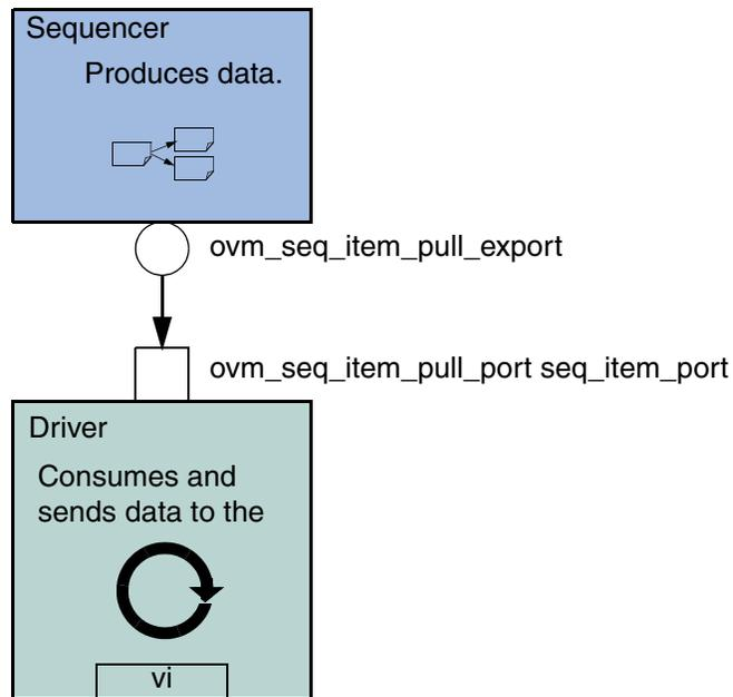
The `seq_item_port` in `ovm_driver` defines the set of methods used by the driver to obtain the next item in the sequence. An important part of this interaction is the driver's ability to synchronize to the bus, and to interact with the sequencer to generate data items at the appropriate time. The sequencer implements the set of methods that allows flexible and modular interaction between the driver and the sequencer.
