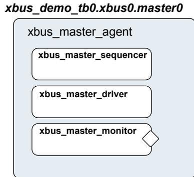
The `build()` function of the `xbus_master_agent` is specified to create the driver, sequencer, and the monitor. The `is_active` property controls whether the driver and sequencer are created.
