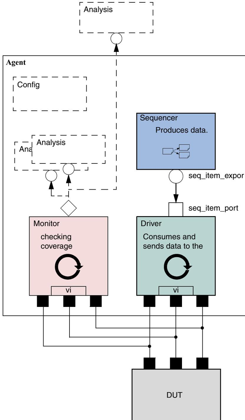
Figure 3-2 on page 37 shows the recommended grouping of individual components into a reusable interface-level OVC agent. Instead of reusing the low-level classes individually, the developer creates a component that encapsulates its sub-classes in a consistent way. Promoting a consistent architecture makes these components easier to learn, adopt, and configure.
