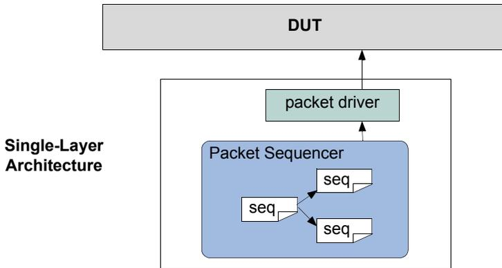
Taking the `higher_layer_item` and `lower_layer_item` example, there is a lower-layer sequence and a higher-layer sequence (complete with their sequencers). The lower-layer sequence pulls data from the higher-layer sequencer (or from the higher-layer driver).
