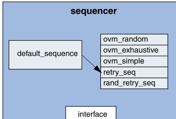
Setting `default_sequence` to "retry\_seq" using `set_config_string("*.sequencer", "default_sequence", "retry_seq");` causes the sequencer to execute the "retry\_seq" sequence.
