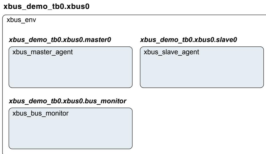
The `build()` function of the `xbus_env` creates the master agents, slave agents, and the bus monitor. Three properties control whether these are created. The source code is shown here.
