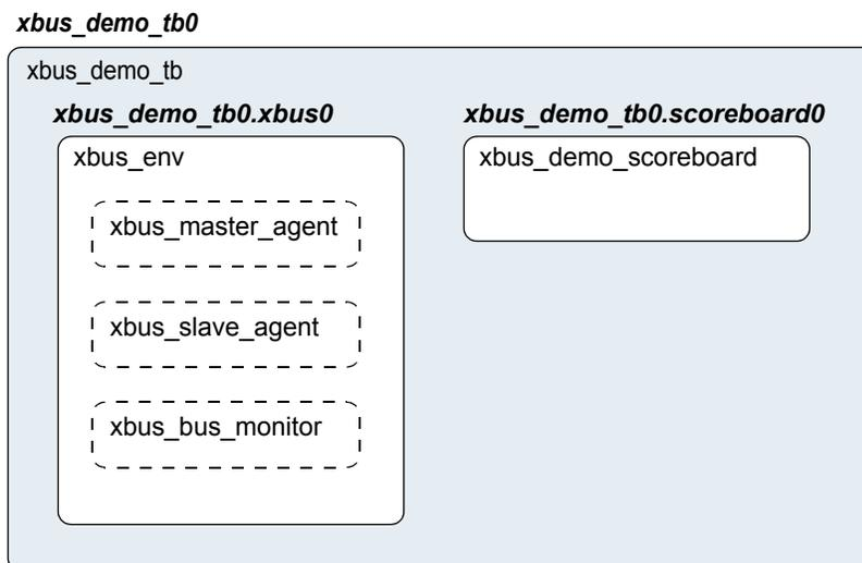
In general, testbenches can contain any number of envs (OVCs) of any type: `xbus`, `pci`, `ahb`, `ethernet`, and so on. The XBus demo creates a simple testbench consisting of a single XBus environment (OVC) with one master agent, one slave agent, and one bus monitor (see [Figure 6-2](#) on page 146). The following code defines a class that specifies this configuration. The test will create an instance of this class.
