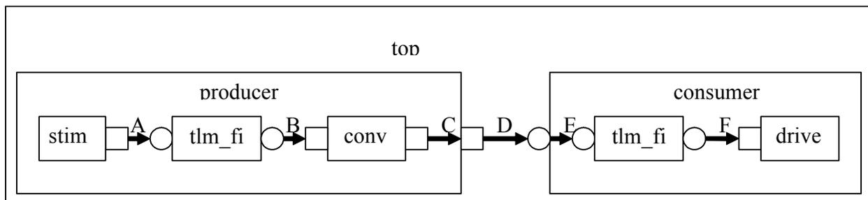
The hierarchy of this design contains two components, `producer` and `consumer`. `producer` contains three components, `gen`, `fifo`, and `conv`. `consumer` contains two components, `fifo` and `driver`. Notice that, from the perspective of `top`, the `producer` and `consumer` appear identical to those in [Figure 2-1](#) on page 21, in which the `producer's`
