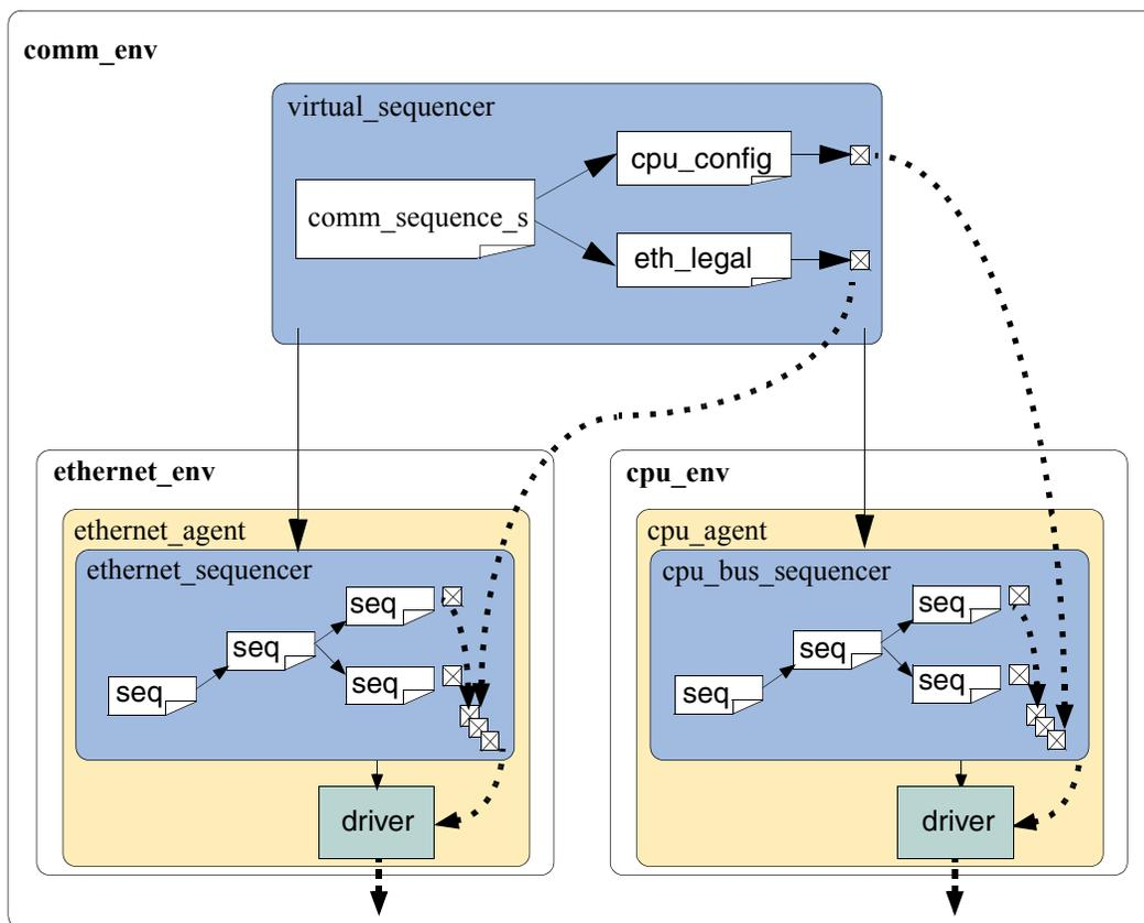
There are three ways in which the virtual sequencer can interact with its subsequencers:
